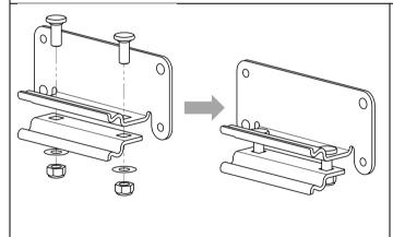
1. Assemble brackets with a pair of M8 Bolts, Washers and Nuts
